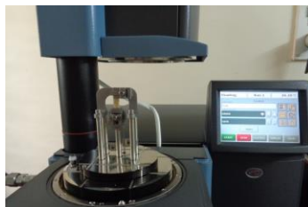
Fig2: DMA TEST RIG
